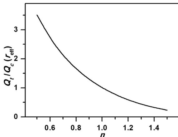
**Figure 6.** Ratio of the flow in a tapered needle  $Q_t$  to the flow in a cylindrical needle with the effective radius  $Q_c(r_{eff})$ , plotted as a function of the power law index  $n$ . For a Newtonian fluid ( $n = 1$ ), flows are equivalent; for shear-thinning fluids ( $n < 1$ ), the flow ratio is greater than 1; and for shear-thinning fluids ( $n > 1$ ), the flow ratio is smaller than 1.
