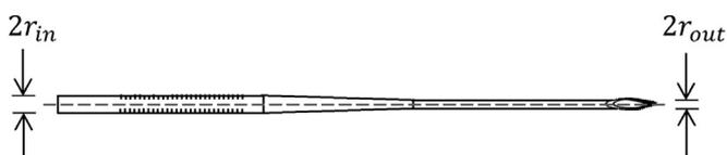
Figure 1. Schematic representation of the 29G TNN.
